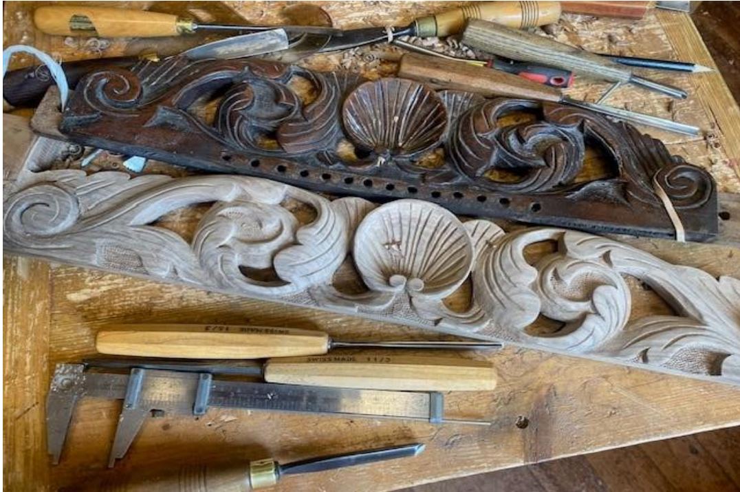
Fig 17, The new carved stretcher with the creating rail as a guide.
